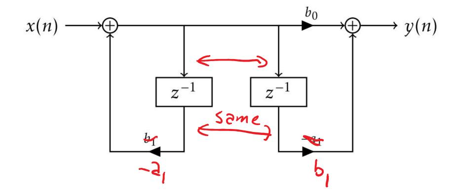
The two delay lines can be merged to direct form II (normal form, canonical form).
