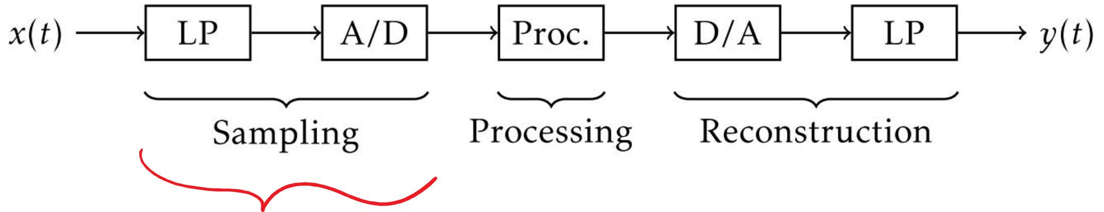
An signal is read at a regular interval
