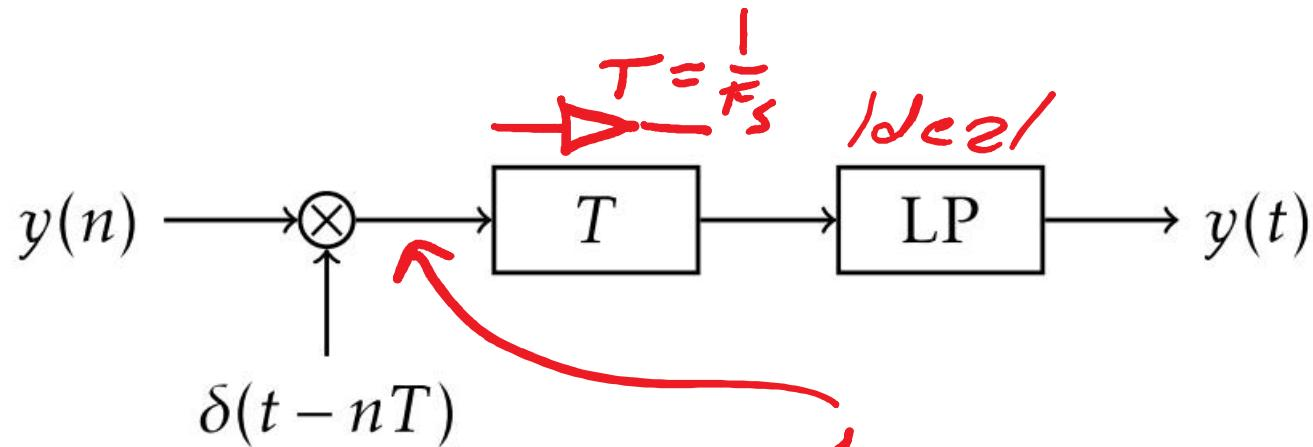
Analog impulse signal of the discrete signal:
