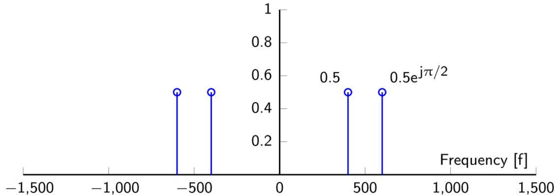
Spectrum after sampling (the discrete signal):
