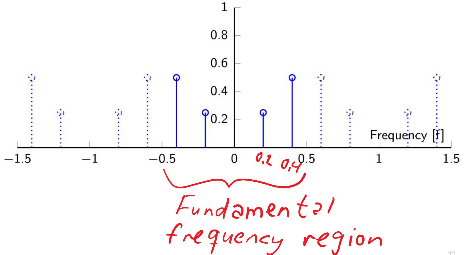
We will avoid aliasing, i.e. any “false” components if we fulfill the sampling theorem, i.e.
